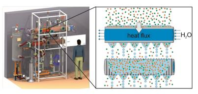
for the heat transfer coefficient on the outside of the condensation tube will be further developed considering influences such as subcooling, surface structure and material composition of the tubes, as well as the thermophysical properties of the refrigerants.
